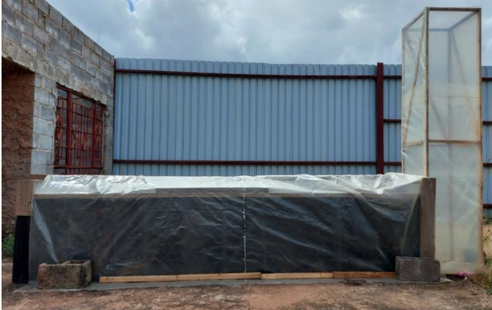
Figure 3.4. A Chimney solar dryer used in drying BSFL.
