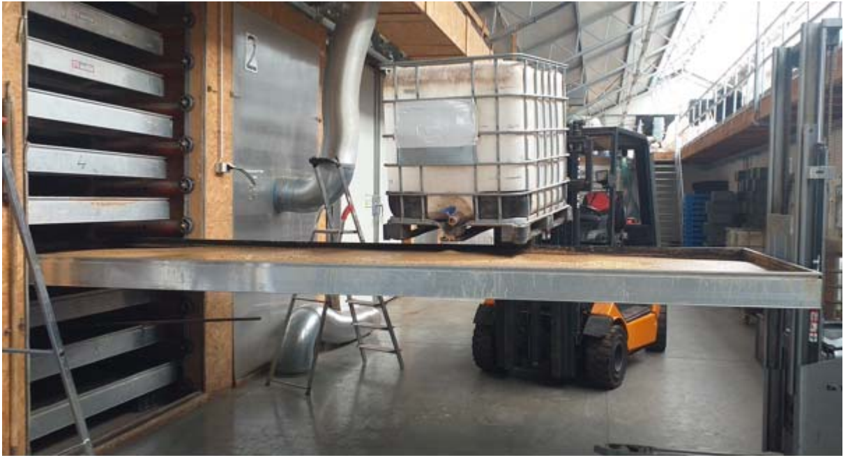
Figure 11: larvae rearing tables/trays with larvae feed ready for rearing.
